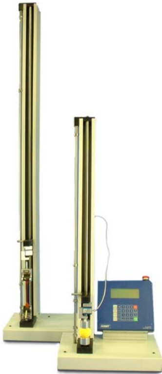
eXpert 7601 and eXpert 7601 extended frame universal testing machines with 1KN (225 Lb) capacity.
