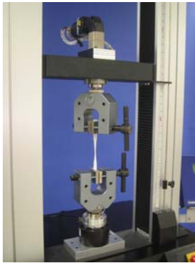
eXpert 2611 outfitted with an optional torsion actuator for bi-axial testing.
