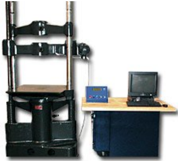
Figure 7: Retrofit of 60,000 lb capacity testing machine with Windows-based system and new servo hydraulic power unit.
