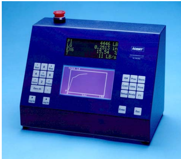
Figure 4: Multi-channel digital indicator capable of calculating the common mechanical properties of metals.
