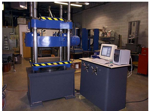
Figure 6: Retrofit of 400,000 lb capacity hydraulic testing machine with Windows-based system and existing manual controls.
