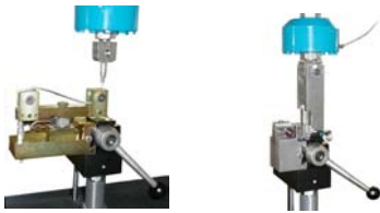
Example of quick change tooling used for performing moment tests.
