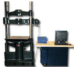
60K Baldwin upgraded with new servo-hydraulic power unit and ADMET's MTESTWindows Materials Testing System.
